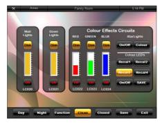
The DMX and Dimming Controls for the Family Room where Colour changing and Lighting levels can be adjusted and stored for quick access from the 5 Scene Buttons.
